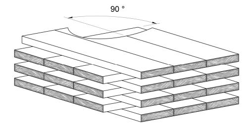
Figure 2: Principle structure of cross laminated timber with 3 layers
